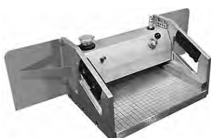
Air Tenon Jig - Travels in 3/4" x 3/8" groove
