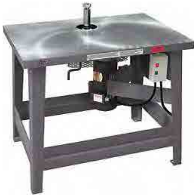
A Shaper 7-1/2 HP (1-1/4" Spindle, 28"x40"top)
