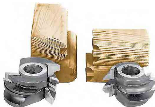
1 3 / 8 " Interior Profile, using one spacer & the 1/4" groover.
