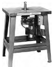
Shaper \frac{3}{4} " Spindle, 20"x28" top w/ Table Top Groove
